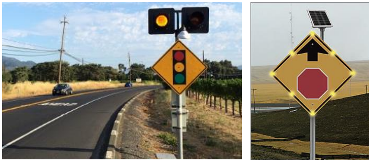
Figure 20: Example of Flashing Beacons or LED Lights as Advance Warning to Intersection
