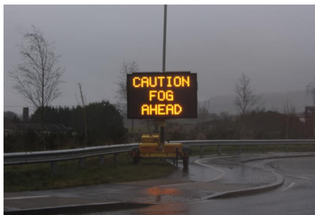
Figure 15: Example of Variable Message Sign
