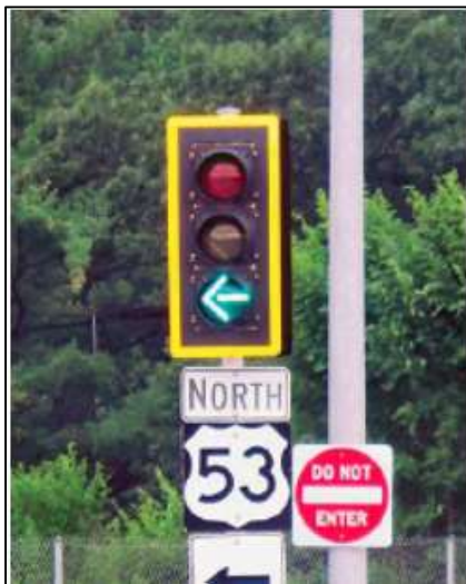
Figure 17: Example of Signal Backplate Framed with a Retroreflective Border
