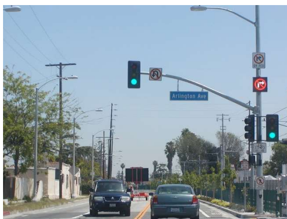
Figure 20: Example of No Right-Turn on Red
