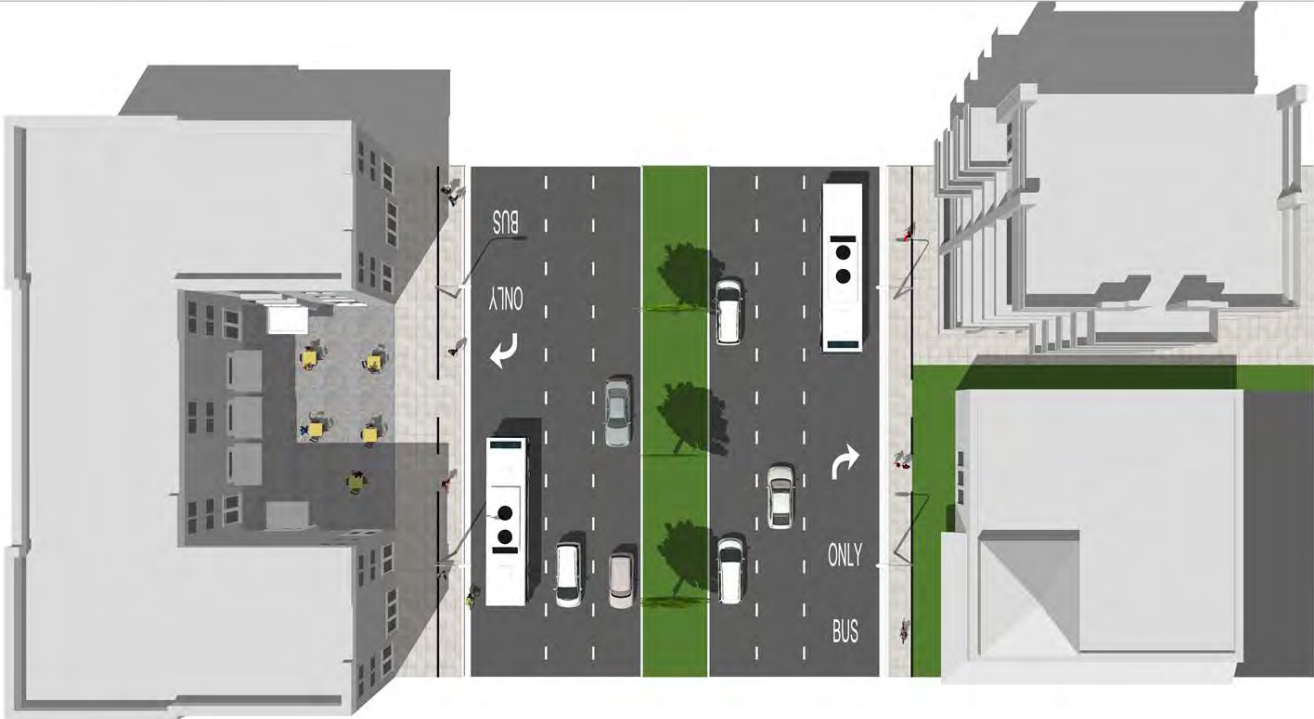
Figure 10: Alternative A aerial showing inconsistent sidewalk width
